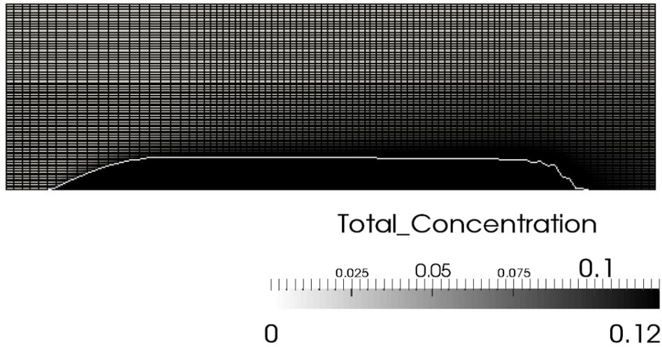
Fig.3 Computational grid, Bed height and concentration distribution at  $t = 8$  s
