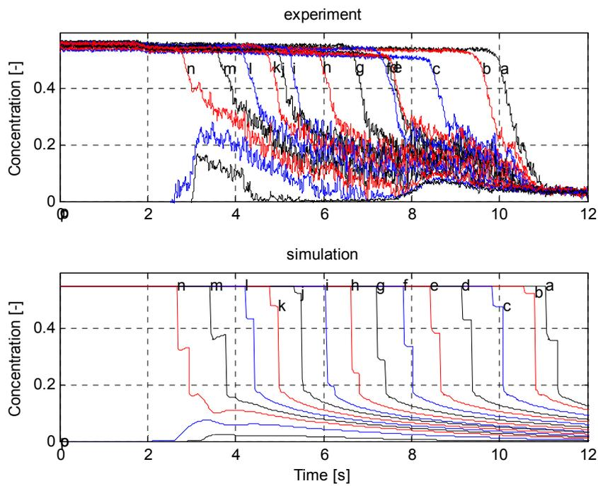
Fig.4 Measured and calculated concentration development
