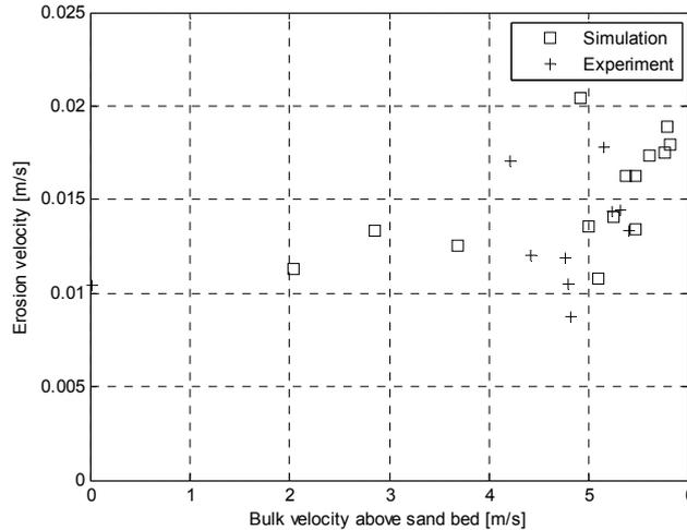
Fig.5 Comparison between the measured and calculated erosion velocity
